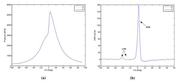
Figure 6: (a) Cylinder pressure versus Crank Angle (b) Heat release Rate versus Crank Angle (C and F refer to engine operating points in Table 2)
