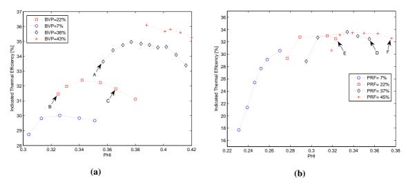
Figure 3: Variation of indicated thermal efficiency versus equivalence ratio at different (a) BVPs and (b) PRFs. (A through F correspond to engine operating points listed in Table 2)
