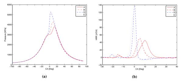
Figure 5: (a) Cylinder pressure versus Crank Angle (b) Heat release Rate versus Crank Angle (A through D refer to engine operating points in Table 2)
