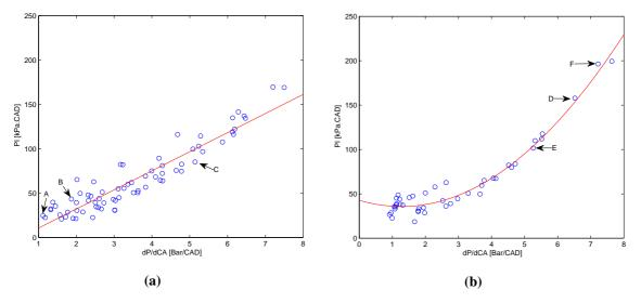
Figure 4: Pressure Intensity (PI) versus maximum rate of pressure rise at different (a) BVPs and (b) PRFs. (A through F correspond to engine operating points listed in Table 2)
