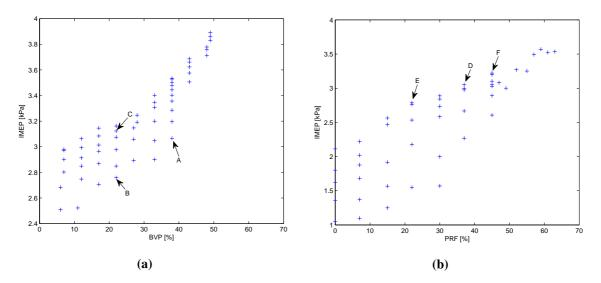
Figure 2: IMEP versus (a) BVP and (b) PRF (A through F correspond to engine operating points listed in Table 2)
