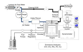
Figure 1: Single cylinder engine testbench schematic
